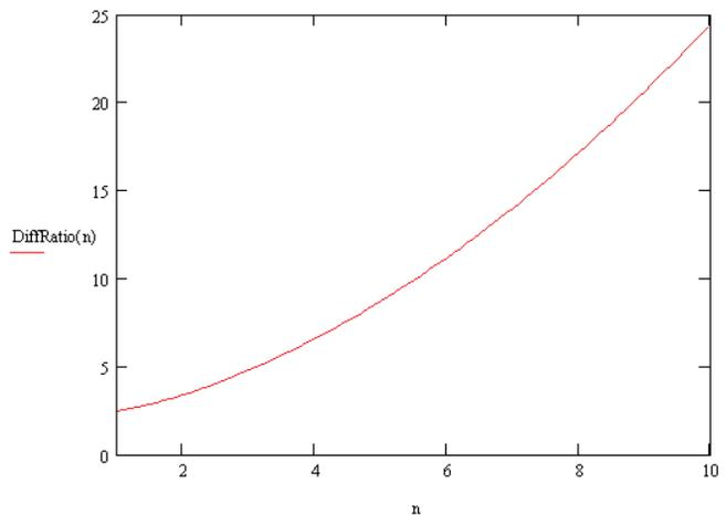
**Figure 6:** The ratio of the coupled noise from a single-ended driver (Trace b) on a single-ended Trace c compared to the noise from a differential pair Trace a and Trace b on another differential pair, Trace c and Trace d (from Eq. 21).
