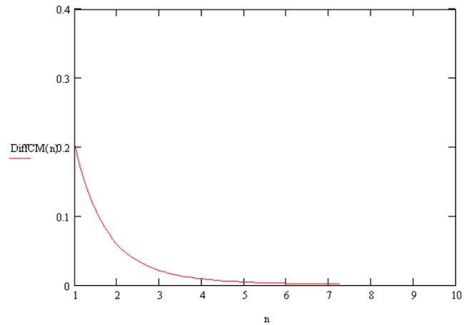
**Figure 5:** The normalized coupled noise on the differential pair, Trace c and Trace d, caused by a differential signal on Trace a and Trace b as a function of n (from Eq. 19).
