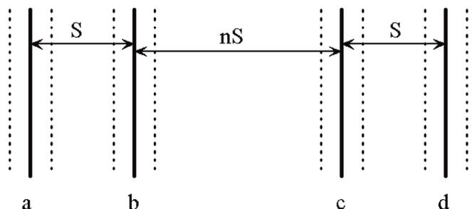
Figure 1: Typical traces on a PCB.
