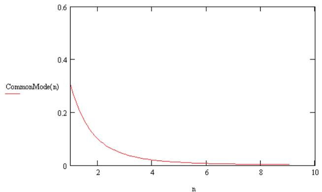
**Figure 3:** The normalized coupled noise on the differential pair, Trace c and Trace d, caused by a signal on Trace b as a function of n (from Eq. 8).
