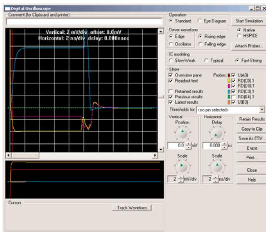
Figure A6 - The coupled crosstalk signals from the model shown in Figure A5.
