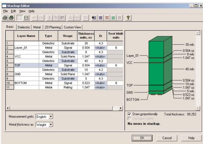
Figure A1b - Typical stackup for deeply embedded microstrip and unbalanced stripline.
