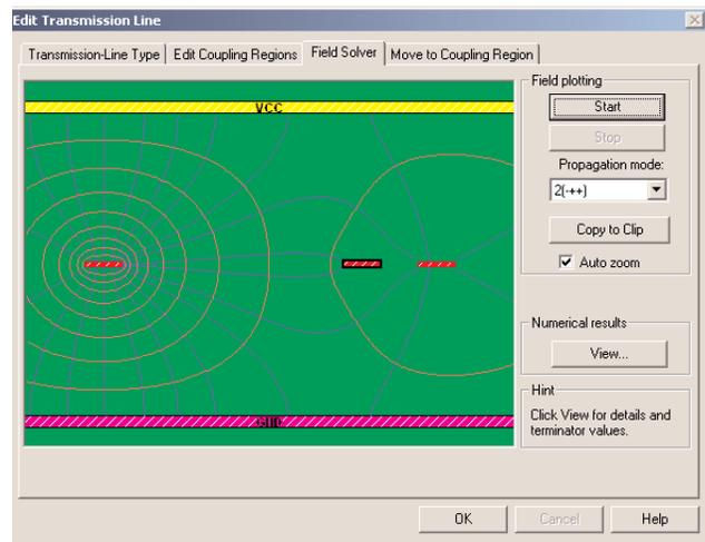
Figure 8 - Representative field solver pattern for Case B, balanced stripline.
