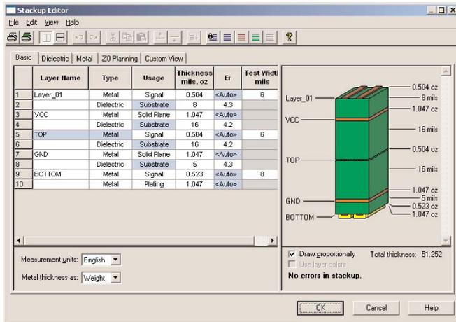
Figure A1a - Typical stackup model for microstrip and balanced stripline.
