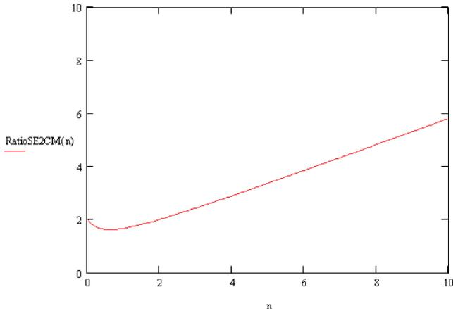
**Figure 4:** The ratio of the coupled noise from a single-ended driver (Trace b) on a single-ended Trace c compared to a differential pair Trace c and Trace d (from Eq. 10).
