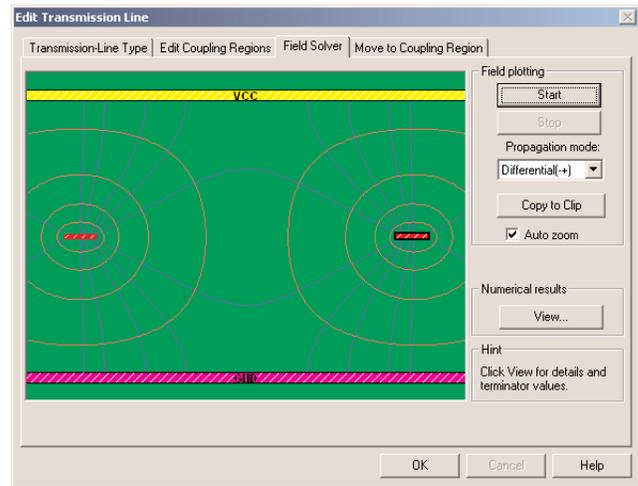
**Figures 7a and b** - Field solver results for 36 mil separation for the embedded microstrip (a, below - left) and for the balanced stripline (b, above) Case A simulations.
