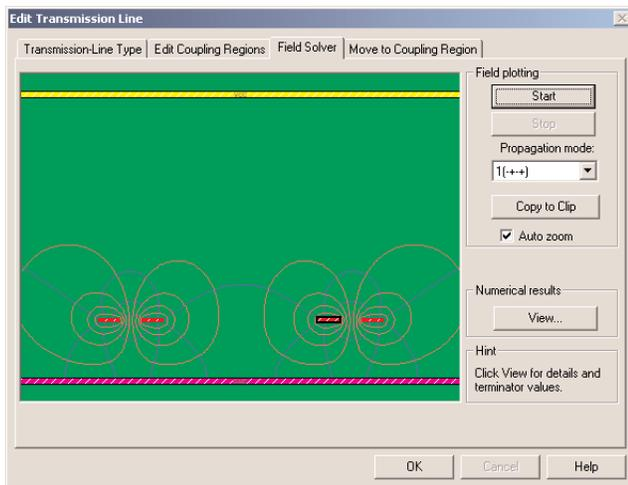
**Figure 9** - Representative field solver pattern for Case D, asymmetric stripline.
