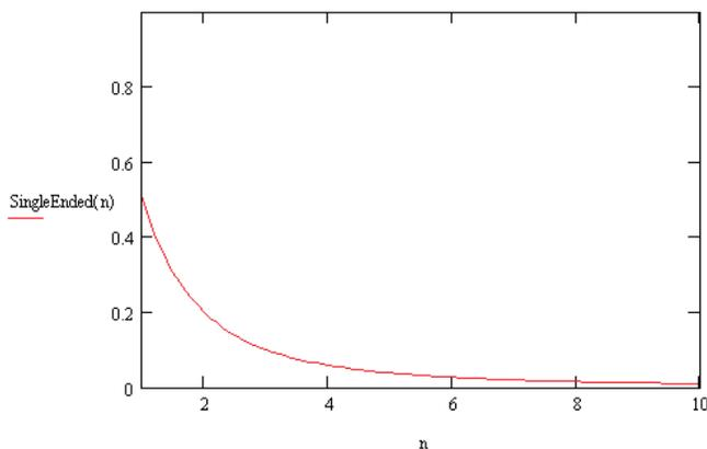
**Figure 2:** The normalized coupled noise on Trace c caused by a signal on Trace b as a function of n.
